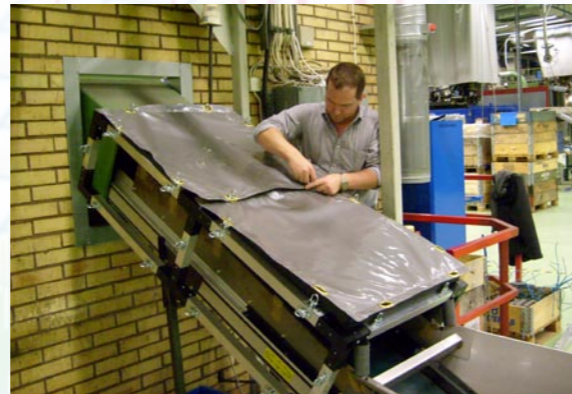
The main areas for Rapid MSS is as sound enclosure for granulators and their transport system.
