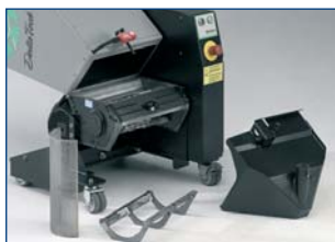
Easy service/cleaning – instant access to rotor and cutterhouse.
