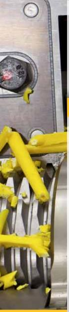
The Rapid RG Series is specifically designed for beside-the-press recycling of hard and brittle materials. The ultraslow rotor speed and screenless operation provides low noise level and very low dust level even with the most filled and brittle materials.
