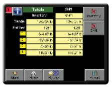
Instantly see your materials usage Material usage / totals screen tracks the number of batches, weights dispensed by bin and weight
