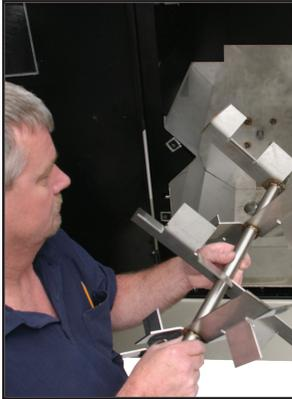
Easy access to all material contact points for fast and safe cleaning during color or resin changes. Material compartment access doors, removable weigh bin, mix agitator and mix chamber liner allow quick efficient cleaning.
