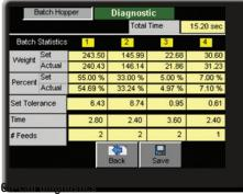
Diagnostic screen displays target set point percentage and actual percentage dispensed. Also displays start and finish weights for each material per batch. Verifies true and accurate blend performance.
