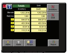
Material usage / totals screen tracks the number of batches, weights dispensed by bin and weight dispensed in total since the last reset.
