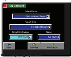
Every SB-2 blender control is equipped with the capability to help users track their settings, alarms, material consumption, shift and inventory needs.
