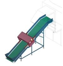
**Easy to install** – The tunnel type metal detector series D feature an upper and lower part that are screwed. This way the tunnel can be separated for installation on the transport system. Alignment bolts ensure that the two tunnel sections are properly positioned after the assembly. The detector is immediately ready for use without the need to re-calibrate. The cable connecting both parts is a plug connection, which saves time and avoids wiring errors.
