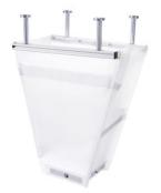
The collecting funnel ATB-G with straight runout is mounted under the tool of an injection moulding machine via strong permanent magnets. It safely collects the moulded parts after demoulding and transfers them onto a conveyor belt or into a container below the machine. The funnel is movable and follows the tool. Optional equipment such as bafflers or a cut-out for conveyor belt ensures damage-free collection and waste reduction of the moulded parts.
