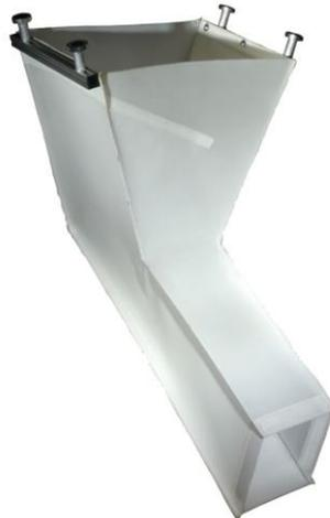
The collecting funnel ATB-S with diagonal runout is mounted under the tool of an injection moulding machine via strong permanent magnets. It safely collects the moulded parts after demoulding and transfers them onto a conveyor belt or into a container next to the machine. The funnel is movable and follows the tool. Optional equipment such as a baffle or a removable base ensures damage-free collection and waste reduction of the moulded parts.
