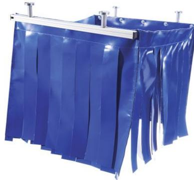
The collecting funnel ATB-L with lamellas is mounted under the tool of an injection moulding machine via strong permanent magnets. It safely catches the moulded parts after demoulding and passes them onto a conveyor belt or into a container below the machine. The funnel is moveable and follows the tool. Cooling or tempering hoses can be passed through the lamellas easily, without new complex placement of the hoses.
