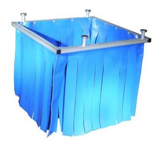
The ATF-L collecting funnel has a fixed frame and is mounted in the bed of an injection moulding machine via strong permanent magnets. The strip fingered side walls mean that cooling or tempering hoses can pass through the funnel, negating the need to re-route them. It safely catches the moulded parts after demoulding and directs them onto a conveyor belt or into a container below the machine.
