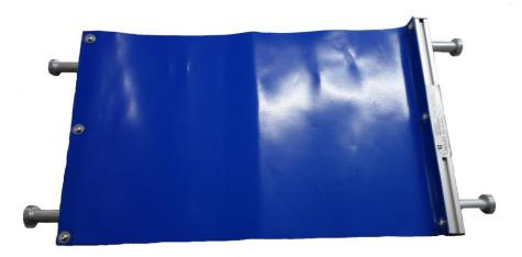
The collecting chute ARB is mounted on the clamping plates and the installed funnel of an injection moulding machine via strong permanent magnets. It safely collects the moulded parts after demoulding and transfers them into the installed funnel of the machine. The chute flexes to move with the tool. This chute closes the gap between the tool and the installed funnel of the machine.
