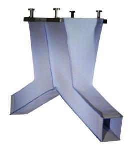
The collecting funnel ATB-DS with two diagonal runouts is mounted under the tool of an injection moulding machine via strong permanent magnets. It safely collects and separates the moulded parts after demoulding and transfers them onto conveyor belts or into containers next to the machine. The fabric funnel flexes to move with the tool. Optional attachments such as soft drop baffler and/or removable base ensures damage free collection and waste reduction of the moulded parts.
