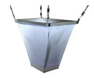
The collecting funnel ATF with straight runout is mounted in the machine bed of an injection moulding machine via strong permanent magnets. It safely collects the moulded parts after demoulding and transfers them onto a conveyor belt or into a container below the machine. The funnel has a fixed frame. Optional equipment such as soft drop bafflers or mounting via brackets ensures damage-free collection and waste reduction of the moulded parts.
