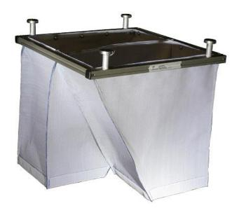
The collecting funnel ATF-D with two straight runouts is mounted in the machine bed of an injection moulding machine via strong permanent magnets. It safely collects the moulded parts after demoulding and transfers them onto conveyor belts or into containers under the machine. The funnel has a fixed frame. Through the two runouts, parts can directly by separated from sprue while falling.
