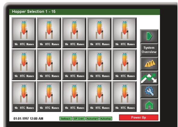
Access to your hoppers, (one or multiple) is just a click or two away from any screen on the DC-T. You can quickly see what is happening in each hopper, identify any issues before they become problems, and change setpoints easily when material changeovers occur.
