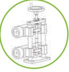
Pinch roll 4-2R (4.12 inch diameter, 2.0 inches wide. Maximum opening 3.0 inches. Single servo only.)
