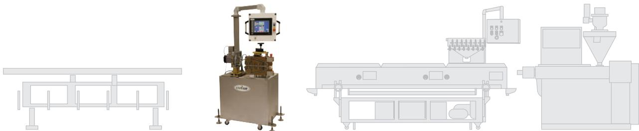
The MedLine is used in-line, downstream from the extruder and tank, to pull, cut, or pull and cut product which can then be transferred to a Medical Take Away Conveyor or coiled onto a Conair ATC coiler.
