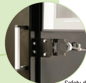
Safety disconnect has been relocated to the outside of the door.
