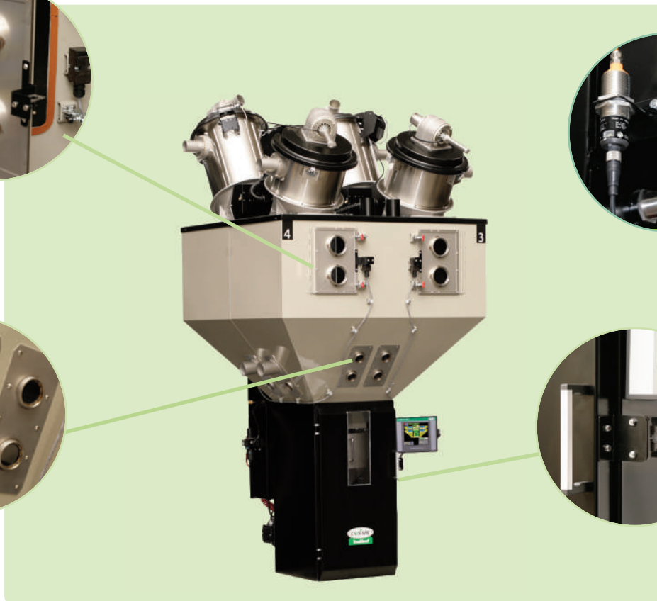
Each access door opening has two round heat-treated sight glasses.
