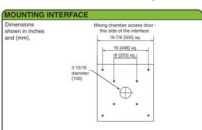
Mounting bolt hole size (8 holes) 9/16 inch {14.0 mm}. Predrilled 8 x 8 and 16 X 16 mounting pattern as standard.
