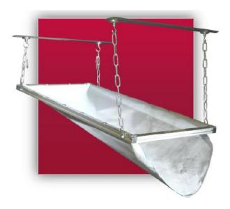
The collecting chute ARF is mounted in the machine bed of an injection moulding machine via strong permanent magnets and chains. It safely collects the moulded parts after demoulding and transfers them onto a conveyor belt or into a container next to the machine. The chute has a fixed frame. In addition, the chute is constructed flat and space saving.
