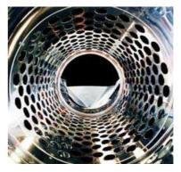
Perforated stainless steel drum especially for round parts separation
